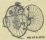
Leading Features. Open front. Rear steering. Left-hand steering. Two speeds.
